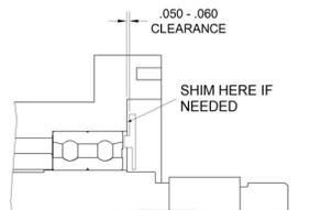
9. Make sure backface clearance is correct. Remove bearing retainers and grease both front and rear bearings through grease fittings until grease is visible around ball assemblies.
